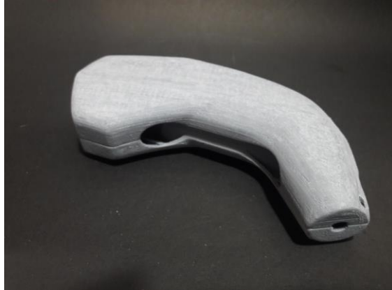
STAGE 1 : FDM PRINTED PART
