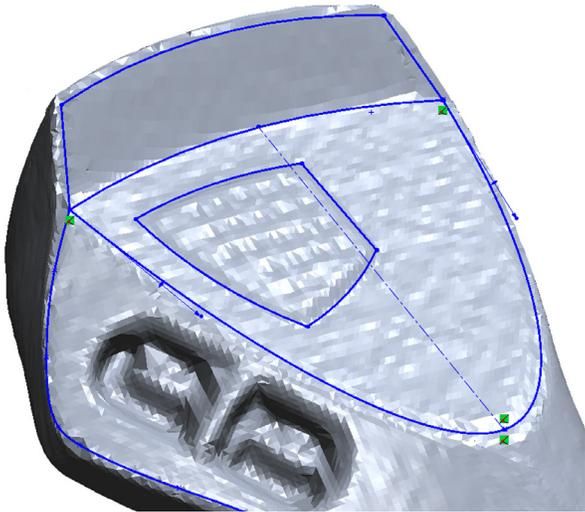
2D and 3D sketches can occur directly on the scanned mesh.
