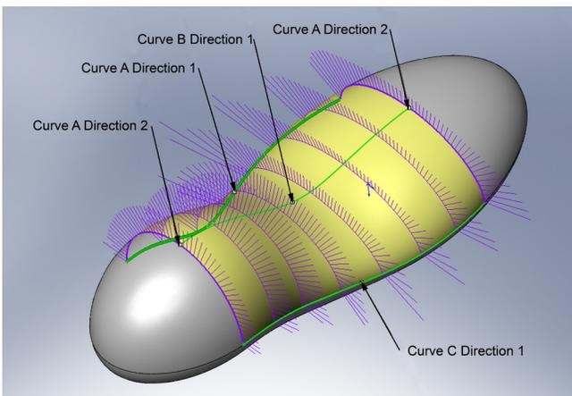
Multiple first and second direction curves can be incorporated with C2 continuity and curvature analysis.
