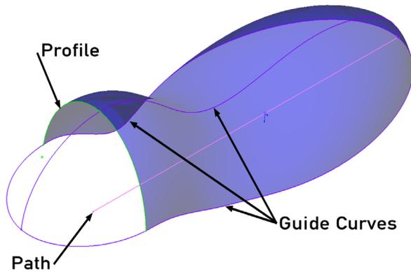
Sweeping with multiple paths, guide curves can easily produce complex shapes.
