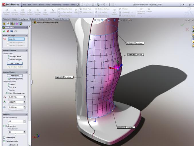
The Freeform feature allows you to place points where you want to pull and dynamically drag the surface to change its shape.
