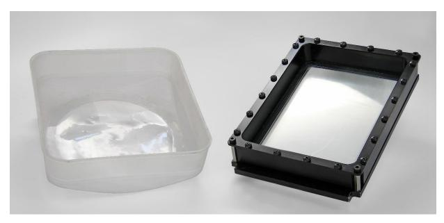
The quality of the material tray used during 3D printing can have a significant impact on the quality and accuracy of the final part, because light must travel through the bottom of the tray to cure an even layer of resin across the build platform. On the left, a used material tray from a budget 3D printer. On the right, a robust material tray from EnvisionTEC that is made with optical glass and an aluminum frame.
