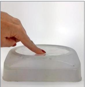
In the image above, a touch from a finger can cause flexible build trays to move, showing how prone they are to distortion during an active 3D print build.
