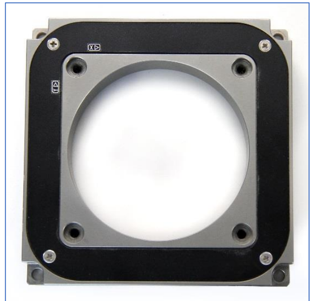
This is a photograph of the EnvisionTEC Enhanced Resolution Module (ERM), which moves a projector, seated in the middle, a half pixel in X and Y, to slightly shift the second exposure in its DLP machines and reduce stairstepping in a sophisticated 3D anti-aliasing technique.
