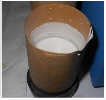
Place flasks in pre-heated 200 °F oven and hold for 3 hours. Ramp up to 1200 °F. @ 800 °F per hour. Hold for 40 minutes. Ramp up to 1350 @ 800 °F per hour and hold for 1 hour. Ramp down @ 500 °F per hour to casting temperature.
