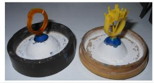
Using a hand piece or jewelers saw, taper the sprue lead as shown to decrease turbulence that may cause investment inclusion during casting.
