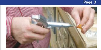
Using the OtoFlash, cure parts on each side using 6500 cycles per side. Rotating the parts cure each side twice for a total of 4 curing sessions.
