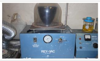
Pour a thin stream of investment to reduce air bubbles. Once the flask is filled place them in vacuum for 45 seconds.
