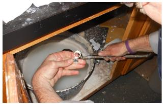
Cast silver part after steam cleaning still connected to button.
