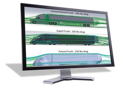
Singley relied on SOLIDWORKS Flow Simulation to run an analysis on the truck and trailer, and determine the actual aerodynamics of the design.
