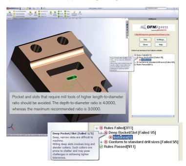
Using SolidWorks CAD software and DFMXpress, you can fully interrogate the manufacturability of your designs to make sure that they are ready to be manufactured. Combined with other SolidWorks Simulation tools, the software can help you build a specialized Design for Manufacturability business.
